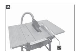
The Rip-Fence (15) has an auxiliary extrusion (27) which has two different guide faces which should be set according to the thickness of the material to be cut. The extrusion (27) should be used according to Fig.14 for thin material (under 25mm workpiece thickness), and according to Fig.15 for thick material (over 25mm workpiece thickness).
