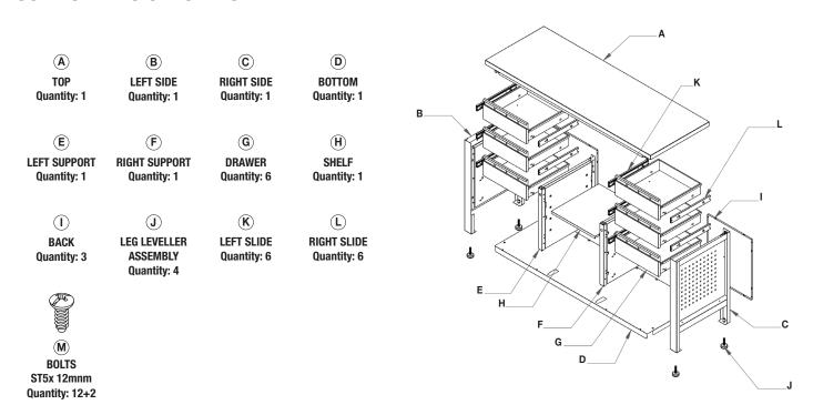
During assembly do not tighten bolts until all components are aligned properly, then tighten fully.
