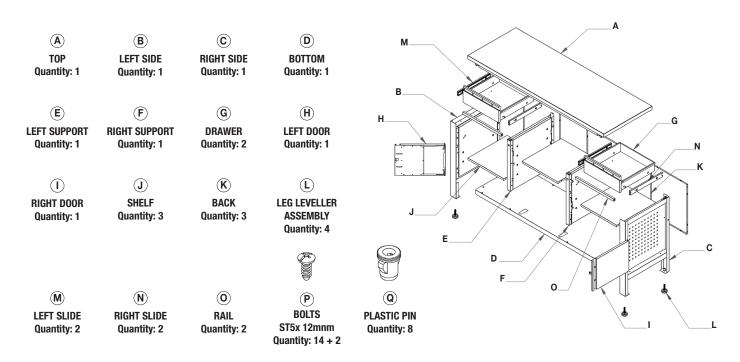
During assembly do not tighten bolts until all components are aligned properly, then tighten fully.
