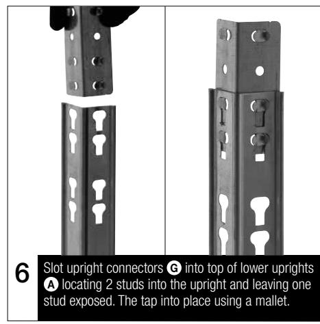
**6** Slot upright connectors **G** into top of lower uprights **A** locating 2 studs into the upright and leaving one stud exposed. The tap into place using a mallet.
