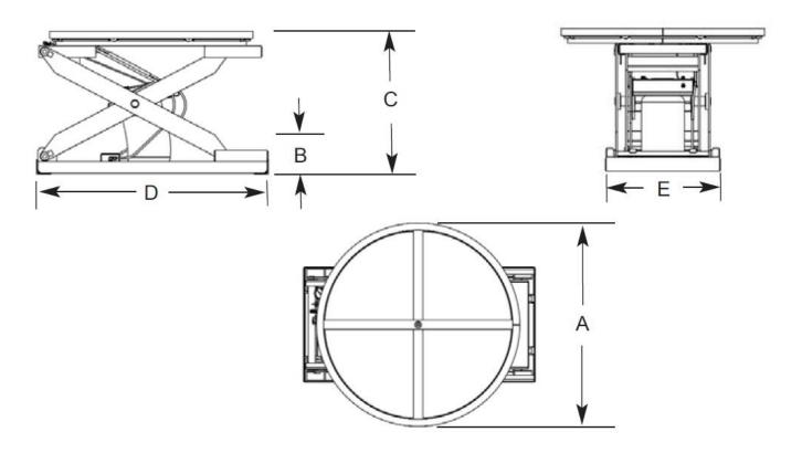
Air Pressure Capacity Adjustment = Infinite (10 - 60 psi / 0.7 - 4.1 bar)On-board Capacity Adjustment = 3 position knob (light – medium – heavy)
