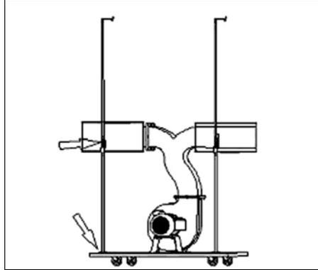
Hang the 2 x filter bags from the upper bag supports and attach to the top of the collectors with the bag clamps. Fit the collection bags to the bottom of the collectors and secure with the other 2 bag clamps.
