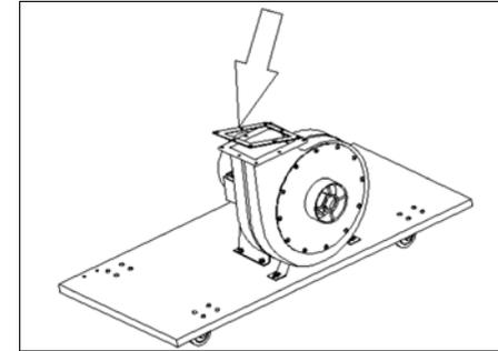
Fit the inlet connector over the gasket ensuring that the holes all line up. Secure in place with the bolts, washers and nuts provided. Fully tighten secure in place. FIG. 4.
