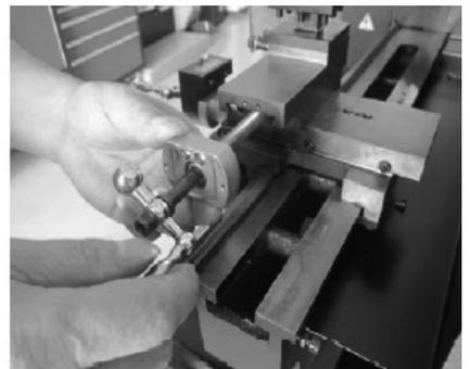
3. Assemble the block (part no.8) and compound feed screw (part no.6) on the bracket (part no.2).
