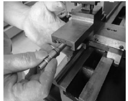
1. Remove the screw securing the compound handle. Remove the ball handle, spacer and dial.
