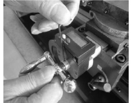
5. Assemble the digital readout box (part no.1) onto the bracket, then fit the assembled transition shaft and ball handle into the leadscrew. Slightly adjust the transition shaft to make it work properly with the leadscrew. Finally, tighten with two M3 x 25mm screws (part no.8).
