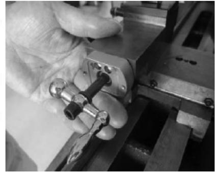
6. Refit the dismantled, original M4 x 12 screws. Take out the transition shaft again.
