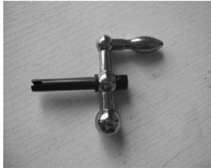
4. Assemble the transmission shaft (part no.4) onto the dismantled ball handle.
