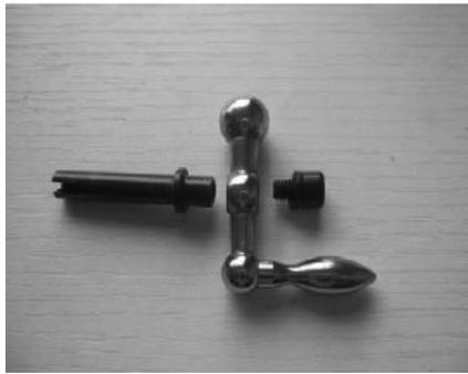
5. Assemble the transition shaft (part no.5) onto the dismantled ball handle.
