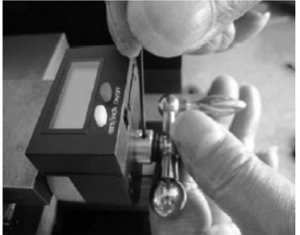
8. Make the final adjustment for free movement of the handle with little drag. Lock the small screws.
