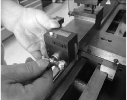
7. Assemble the digital readout box (part no.1) onto the bracket, then fit the assembled transition shaft and ball handle into the lead screw. Slightly adjust the transition shaft to make it work well with the leadscrew. Finally tighten with two M3 x 25 screws (part no.8).
