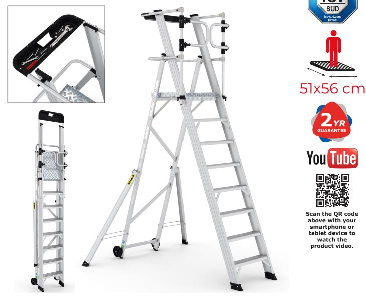
Certified to EN 131 Professional Non-slip aluminium platform 100mm wide treads with non-slip surface to prevent slips Non-slip feet Easily folded & mobile using wheels on rear of product Maximum load capacity of 150kg
