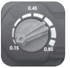
The delay can be adjusted by turning the dial clockwise to either 0.1 fast or 0.8 seconds for a slower delay time.
