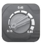
The delay can be adjusted by turning the dial clockwise to either 0.1 fast or 0.8 seconds for a slower delay time.
