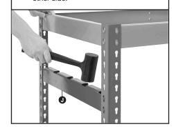
9 Insert Reel Bar (6 into Reel Support Bars
