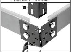
Insert a short side beam into the top two keyholes on the uprights and knock into place using a rubber mallet. Repeat with second short side beam on other side of product
