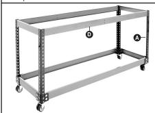
Locate centre support beam fonto the metal studs on the centre of each front and back 'C' section beam for the into place using a rubber mallet.
