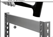
Place front and back 'C' section beams **©** into two remaining top two keyholes on uprights **@** and knock in place with a rubber mallet.
