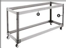
Locate centre support beam onto the metal studs on the centre of each front and back 'C' section beam . Knock into place using a rubber mallet.
