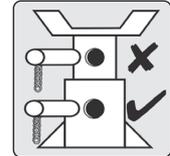
Fit pin through both the stands collar and the centre tube
