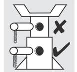
Fit pin through both the stand collar and the centre tube
