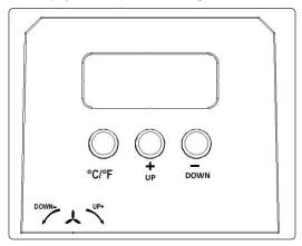
4.7.1. Press the button "+(UP)" or "-(DOWN)" to adjust the temperature.
