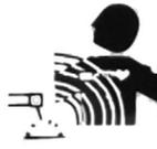
Electromagnetic fields can cause pacemaker malfunction
