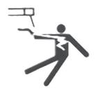
Electric shock from welding electrodes can kill
