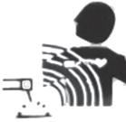
Electromagnetic fields can cause pacemaker malfunction
