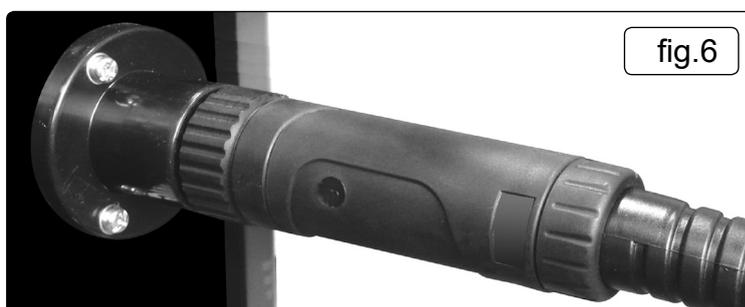
4.8. **CONNECT THE TORCH CABLE TO THE WELDER.** Align the pins on the Euro connector with the socket on the welder front panel as shown in fig.5. Push the connector into the socket and rotate the locking ring (A) clockwise so that it draws the plug into the socket as shown in fig.6.
