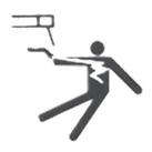
Electric shock from welding electrodes can kill
