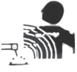
Electromagnetic fields can cause pacemaker malfunction
