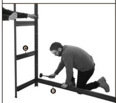
Add remaining Front & Back Beams to the side frames to create the rest of the levels. Ensuring all beams are at the same height.
