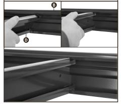
Centre Support ① can be adjusted along shelf level to allow for heavy loads.
