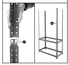
Add remaining side beams **②** and front and back beams **③** to uprights **③** to create the rest of the shelves at the preferred heights.
