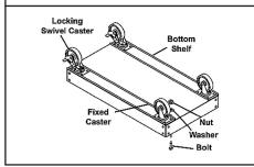
Attach two Locking Swivel Casters to the other side, using eight sets of Bolts (1), Washers (1) and Nuts (2).
