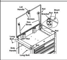
Attach Lid Handle @ using two Screws @.
