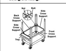
On the same side as Swivel Casters, attach a Side Panel and Tray to the outside, and a Side Cross Support to the inside of Posts using two sets of Long Bolts and Nuts 4.
