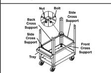
On the other side, attach the remaining Side Cross Support and Side Panel to the inside of Posts using two sets of Bolts and Nuts and Nuts
