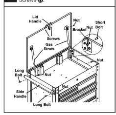
Place one Bracket ® in each corner of Chest. Attach Posts to chest using fourteen sets of Bolts ® and Nuts Ø.
