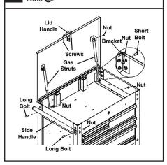
12 Tighten all hardware, starting at the bottom.
