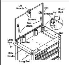
Attach Gas Struts (9) using four Nuts (2).
