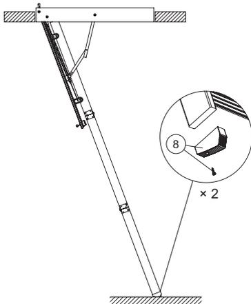
Fully extend the ladder. Ensure the ladder feet rest firmly on the floor and that the treads are horizontal.
