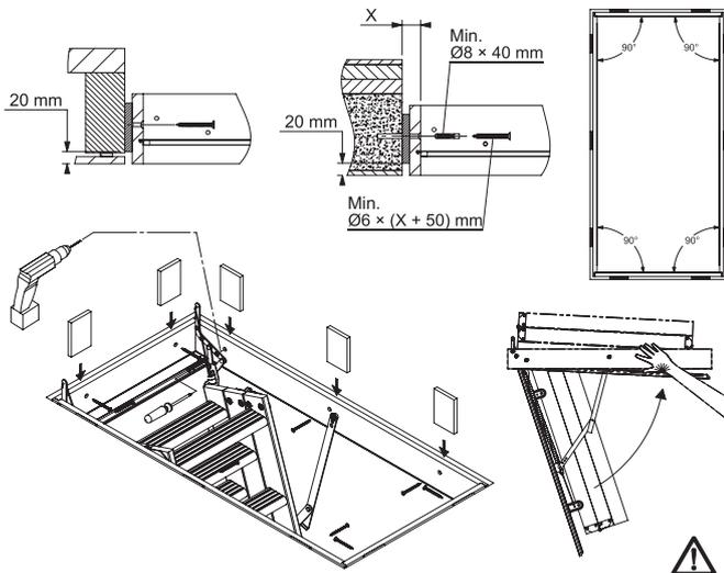
Fit the casing surround to the hatch opening. Ensure the ladder is flat, level and square before fixing.
