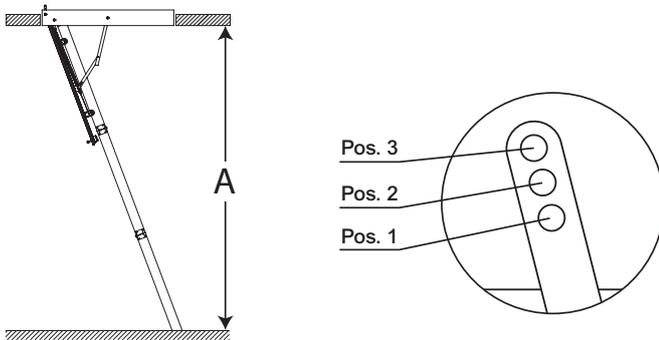
**B)** Use the position calculations to fit the support arms onto the loft casing.
