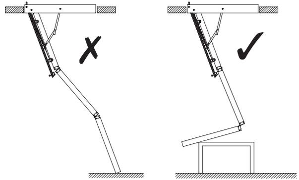
**B)** Measure the ladder section length required and mark this on both sides of the bottom section of the ladder.
