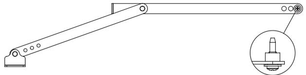
**5** Hinge Clip / Ladder Locking bracket x1
