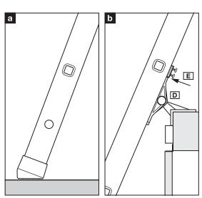
13. Adjusting the Loft Ladder. This adjustment should be done by two persons to avoid climbing the ladder before the stops are locked in position.
