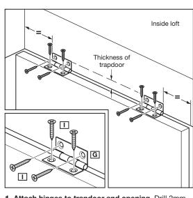
1. Attach hinges to trapdoor and opening. Drill 2mm pilot holes, attach hinges (G) to trapdoor and surround using 8 x csk 20mm screws (I). Note: The trapdoor will attach to the same side of the opening as the ladder (Trapdoor is not supplied).
