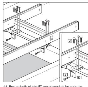
11. Ensure both pivots (D) are spaced as far apart as possible (up against the glides). Use a bradawl or small drill to start the screw holes, attach the pivots to the trapdoor surround using 10 x 25mm screws (J).
