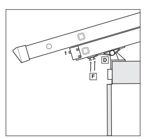
14. Release the locking catch on the top ladder section (1) and slide the bottom section up until it locks. Use the pole to fully stow the ladder. The ladder should not rest horizontally. With the ladder fully stowed, slide the retainers (F) up to the glide/pivot assembly (D) and clip onto the glide.
