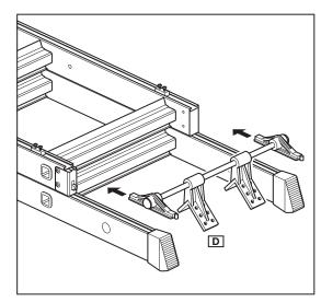
8. Slide the glide/pivot assembly (D) into the ladder, ensure it is fitted the correct way around as shown.
