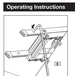
15. To lower ladder. Insert the pole (B) into the round hole on the bottom ladder section and carefully pull down until top section rests on top stops IMPORTANT: Control the movement of the ladder at all times. DO NOT allow ladder to fall under its own weight.
