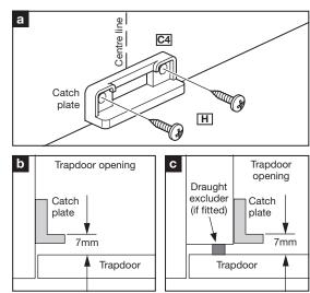
4. Attach catch plate. Find and mark the centre line onto the opening end of the trapdoor surround. Allow a 7mm gap between the top of the catch plate and the trapdoor (b or c). Attach the catch plate (C4) to the trapdoor surround using 2 x 12mm screws (a).
