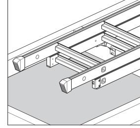
12. Close the ladder, engage the locking catch and slide the ladder into the loft so that the top section is resting horizontally on the loft floor.
