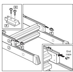
9. Loosely insert 12mm screws (H) into both retainers (F) and slide into the ladder. Refit both end caps.
