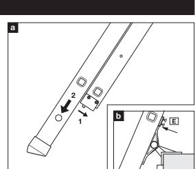
16. When ladder comes to a stop, release catch on top section (1) and lower bottom section (2) until it locks into place (a). IMPORTANT: Ensure top stops (E) are tight
