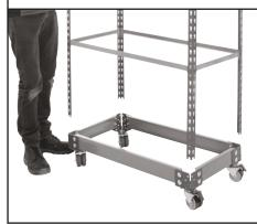
Secure uprights (a) to brackets using four M6 bolts and nuts with a 10mm spanner, placing the M6 washers onto the nut side of the fixing
