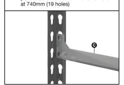
6 Knock beam into position and then repeat step 5 to fit another beam **6** at the same height on the frame. Join beam ends to the second frame as below
