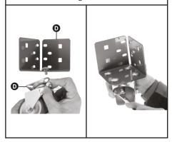
Attach a side 'C' section beam to a bracket using two M10 bolts and nuts with a 15mm spanner, placing the M12 washer onto the bolt side of the fixing
