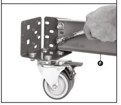
Continue joining side 'C' section beams
