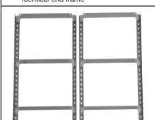
Take a long tyre support beam **©** and insert into the keyholes on one frame with the V profile uppermost as in picture below. Position the lower level
