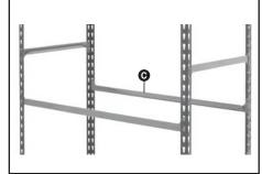
Before adding next tyre beam level, check the height required to allow tyres to be loaded. Then add next two beams as in steps 5 and 6
