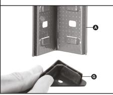
Insert tabs on a side beam 6 into an upright A at preferred height for bottom shelf. Knock into place using a rubber mallet
