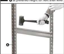
Insert upright connectors • into top of uprights (A) and knock into place using a rubber mallet
