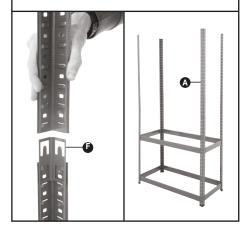
Add remaining side beams **©** and front and back beams **®** to uprights **A** to create the rest of the shelves at the preferred heights
