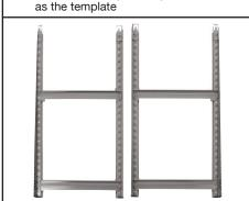
Join the two side frames together using the longer front and back beams B. Ensure front and back beams are positioned at same height as the side
