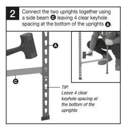
Create two side frames by adding side beams to the uprights as per the below picture. Ensuring side beams are at the same height on each frame. Knock into place using a rubber mallet.
