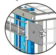
Fix the long brackets on the side perforations of the frames
