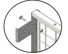
Pre-assemble the long brackets on the back panels before placing the panels on the shelving
