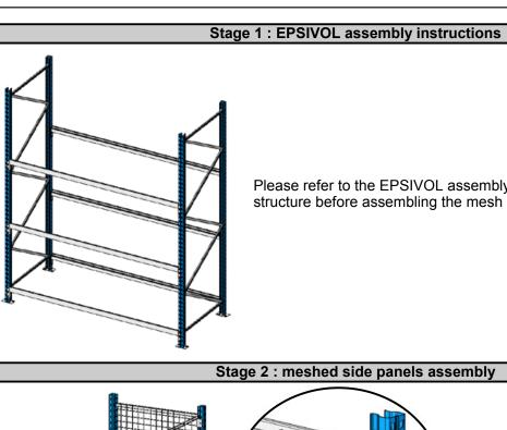
Please refer to the EPSIVOL assembly instructions to built the shelving-structure before assembling the mesh structure
